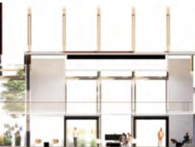
TRUSSES EXPOSED OVER ENVELOPE
